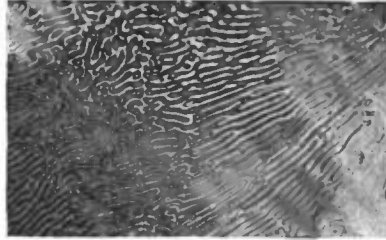
FIG. 2.—(Ewing & Rosenbain, Phil. Trans. ) Lead-tin eutectic. Magnified 750 diameters.
