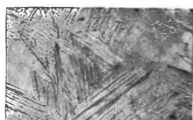
FIG. 11.—(Osmond.) Pearlite steel (carbon about 1%) forged and annealed at 800° C. Magnified 1000 diameters.
