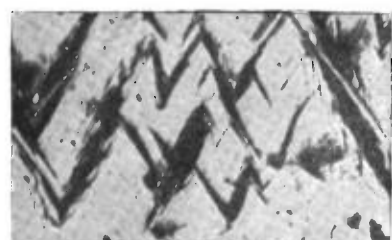
FIG. 15.—(Osmond.) Martensite (black) in austenite (white). Steel (carbon about 1.5%) quenched at 1050° C. in ice-cold water. Magnified 250 diameters.
