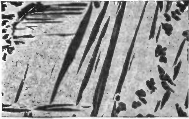
FIG. 1.—(Heycock & Neville, Phil. Trans. ) Bronze containing 23.3% of tin. Slowly cooled. Magnified 18 diameters. Dark parts are rich in copper, light parts in tin.
